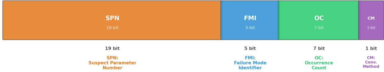
J1939 Diagnostic Trouble Code (DTC) Structure - 32-bit
